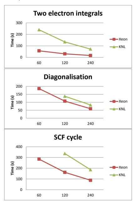
The Scalapack calls in the diagonalisation routine perform almost as well on the Xeon Phi as on Archer, but this is not true of the rest of the code.
