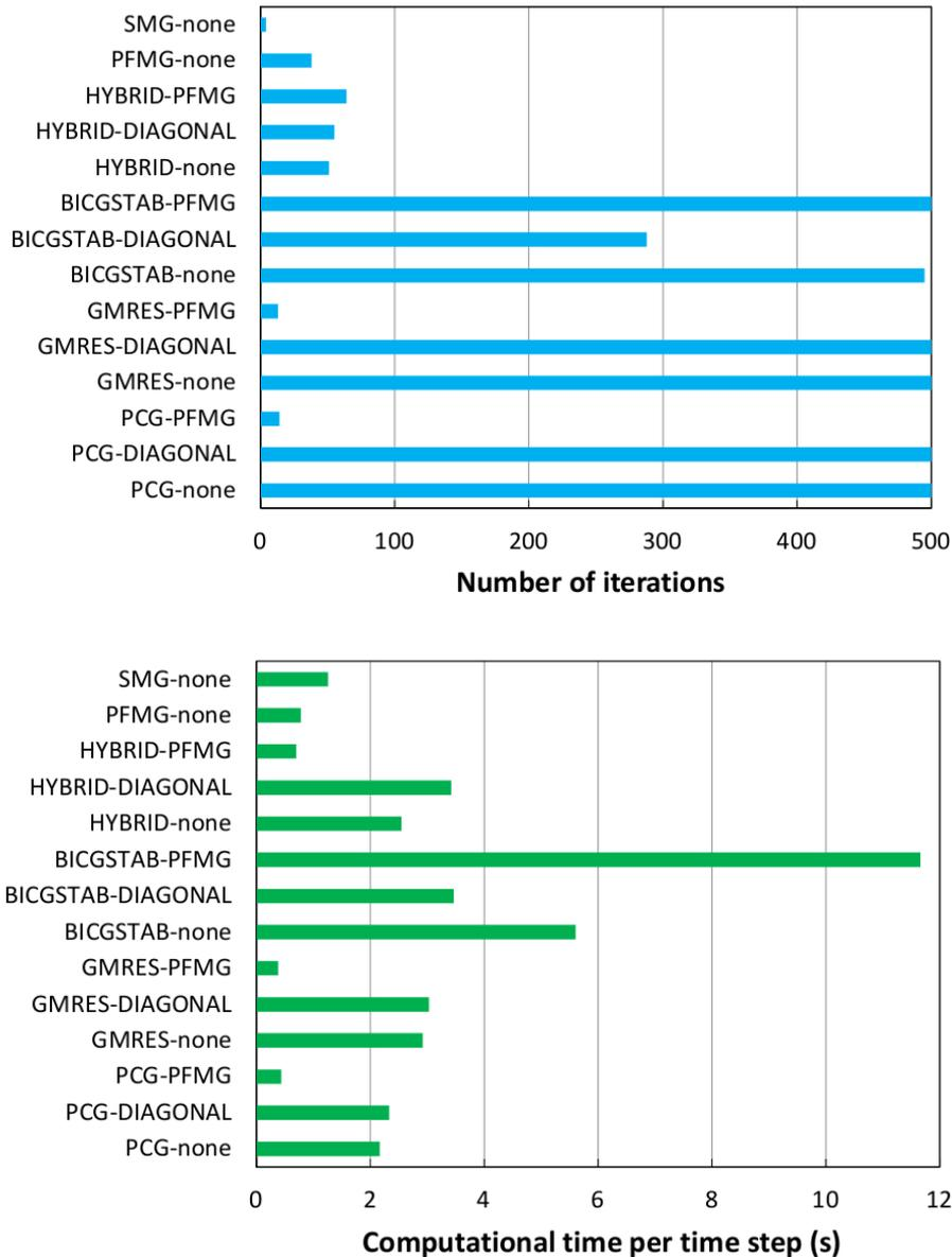
Figure 2. Number of iterations and computational time per time step of the pressure module with various solvers and preconditioners.
