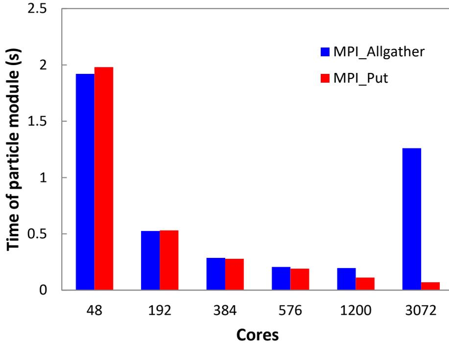
Figure 10. Comparison of the average computational time per time step of the particle module using the MPI collective communication function MPI\_Allgather and the MPI one-sided communication function MPI\_Put.
