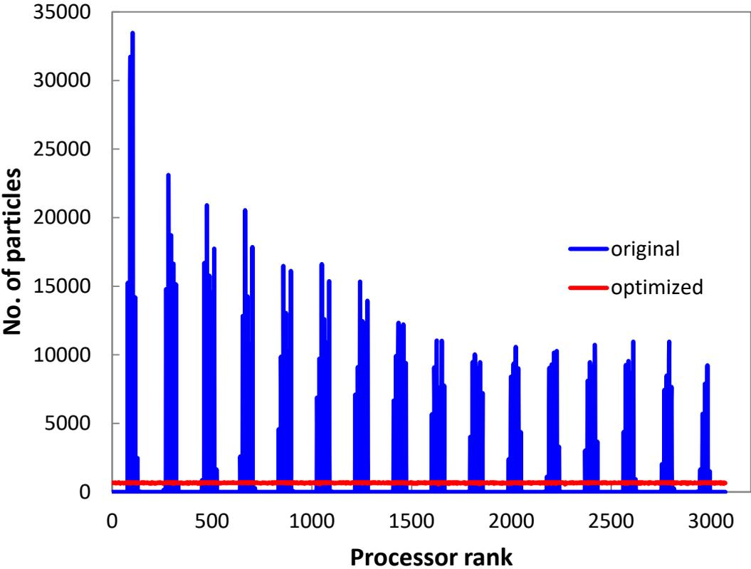
Figure 8. Comparison of the number of particles loaded in each CPU core in the original method and the optimized method.
