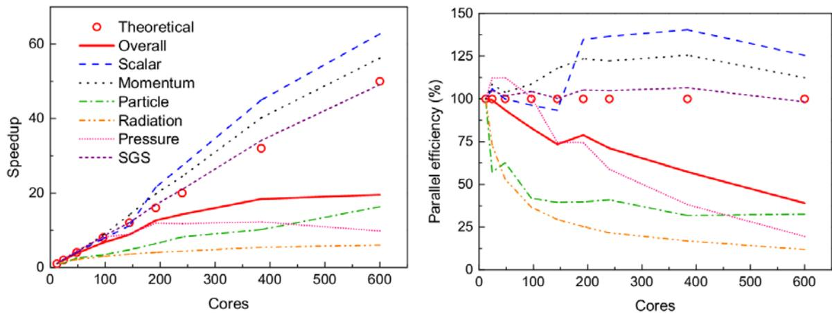
Figure 1. The scaling performance of LESsCOAL on ARCHER before optimization: speedup (left) and parallel efficiency (right) vs. number of cores.
