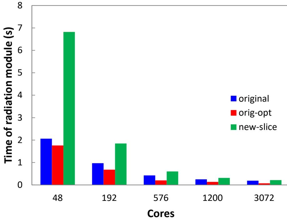
Figure 6. The comparison of the average computational time per time step of the radiation module using different number of cores in the original method, the optimization method 1 (orig-opt) and the optimization method 2 (new-slice).
