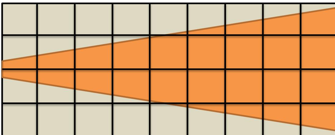
Figure 7. Schematic diagram of the load imbalance issue when domain decomposition strategy is employed for a gas-solid two-phase jet.
