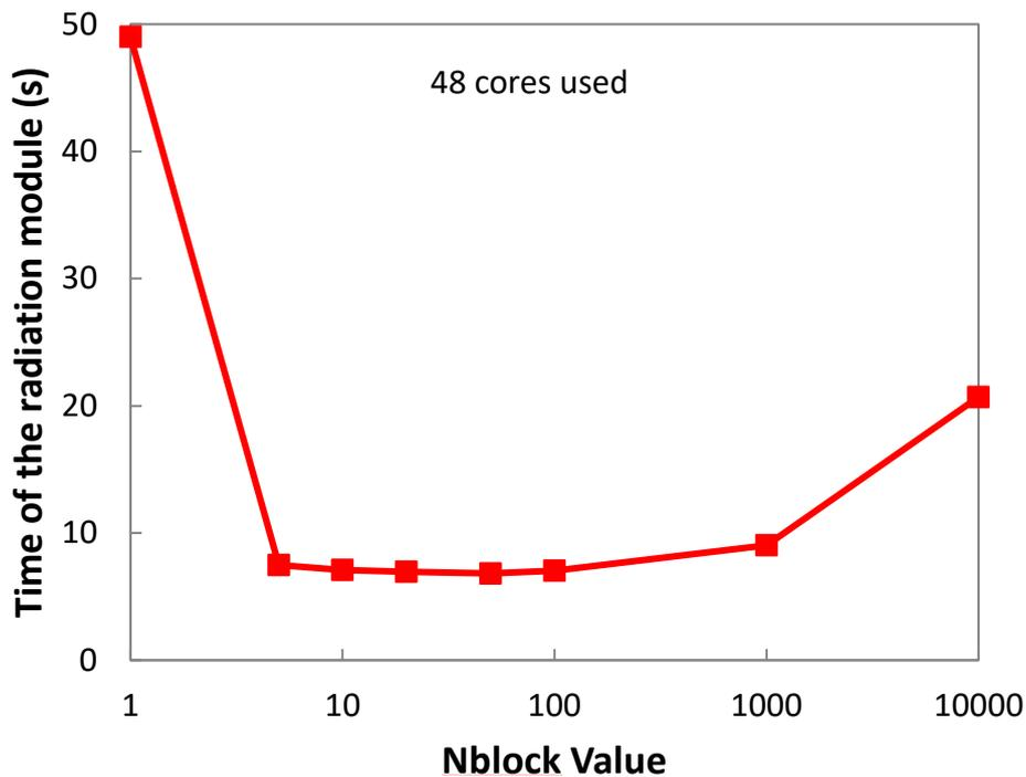
Figure 5. The average computational time per time step of the radiation module with different Nblock values in the diagonal slicing method.
