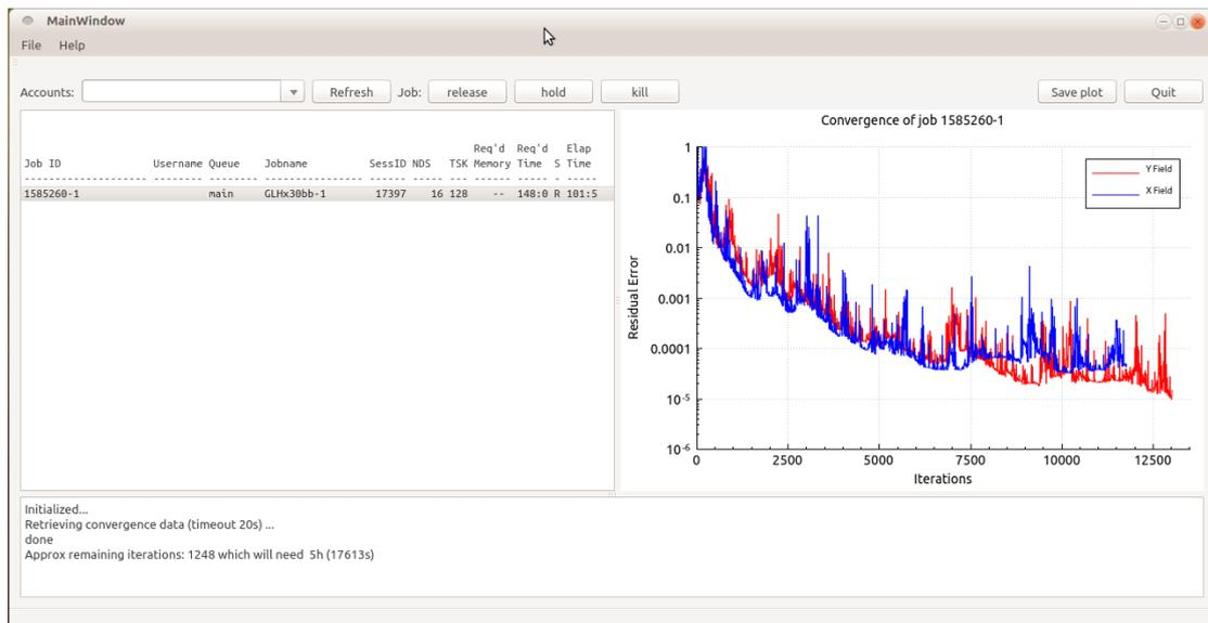
**Figure 1 - Job monitor. The left panel shows Adda jobs on the currently selected remote or local machine. The right panel provides realtime information on the status of the convergence of the computation.**
